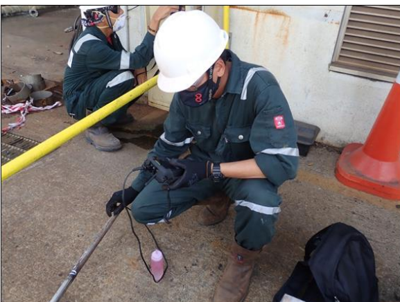
Thickness measurement on defected tube.
